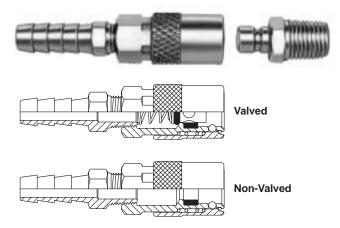
Hansen's Flo-Temp Series provides maximum flow required to cool injection molds. The product is available valved or non-valved depending on your application for use with hot oil, water-glycol, and hot water.
