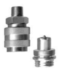
The Series WA 56000 is a high pressure hydraulic screw together coupling designed to operate at pressures up to 10,000 psi.
