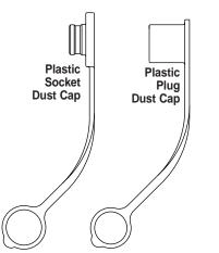
Dust Caps are available where protection is necessary against excessive flying grit or dust. The Socket Dust Cap is easily applied by pulling back the sleeve of the Socket and inserting the Dust Cap. The Plug Dust Cap covers the entire machined surface of the Plug. It is applied and held in place by friction on the locking portion of the Plug. Metal Dust Caps are supplied with chain and attachment ring. Plastic Dust Caps have integral plastic strap and attachment loop.
