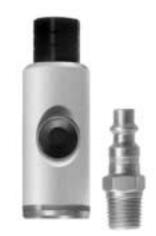
The SAFELINE Industrial Interchange pushbutton safety coupling is safe and easy to connect and disconnect. Twostep disconnect procedure shuts off air supply and releases downstream air pressure before plug can be removed from the socket preventing hose whip.
