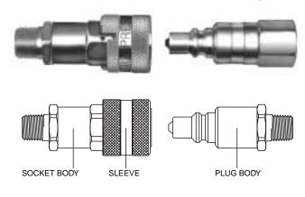
Hansen Series UP (Ultra Pressure) is designed for applications where hydraulic fluid is being used at pressures up to 10,000 psi (700 BAR). The coupling has a ball lock mechanism that replaces the threaded connections typically used in high pressure hydraulics.
