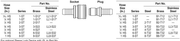
For optional Sleeve Lock Device add -SL to Part No. \*May differ from drawing and is made for hex stock.
