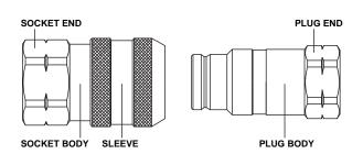
Hansen Series DB is designed for fluid handling where no spillage is required. The coupling is made of 316 Stainless Steel which allows for use in chemical processing, pharmaceutical and food processing industries.
